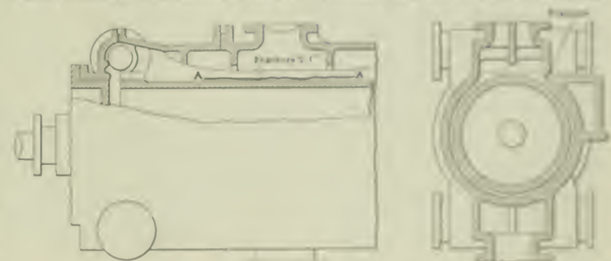
FIG. 3 LONG CRACK IN VALVE CHEST
